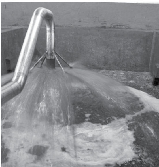
Figure 19.3 Examples of red wine fermentation showing (a) 5 tonne open fermenters, which can be lifted by a crane and taken to a press, (b) 60 tonne rotary fermenter, (c) 50 tonne closed static sweeping arm Potter (SWAP) fermenters, (d) 6 tonne concrete open fermenters with cap submerged using “heading down” boards, and (e) a “pump over” to wet the cap in an open fermenter
