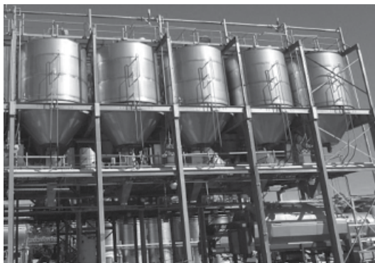
Figure 19.3 Examples of red wine fermentation showing (a) 5 tonne open fermenters, which can be lifted by a crane and taken to a press, (b) 60 tonne rotary fermenter, (c) 50 tonne closed static sweeping arm Potter (SWAP) fermenters, (d) 6 tonne concrete open fermenters with cap submerged using “heading down” boards, and (e) a “pump over” to wet the cap in an open fermenter
